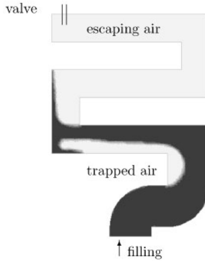
Figure 2. Filling of an S-shaped cavity. The air in the upper part of the cavity is free to escape from the valve. The air trapped by the liquid may exert a force on the liquid, this being neglected in our model.
